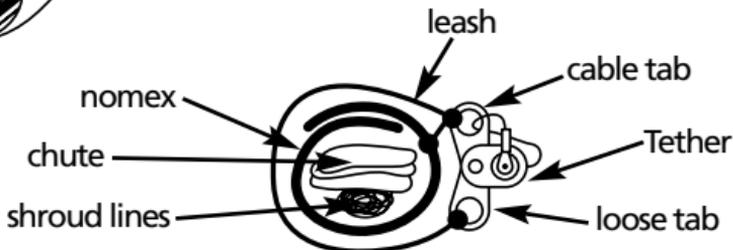
Make a short leash out of nylon or kevlar long enough to reach around the "burrito" with slack. Tie one end to the loose tab. Wrap around and tie to the other tab (with the cable going through it) leaving a little extra tail. Tie the tail to the nomex so you don't lose it.
